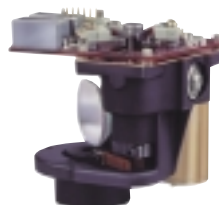
ARMORED PERSONNEL CARRIER Line of Sight Change Rotary Actuator/Mirror Assembly
